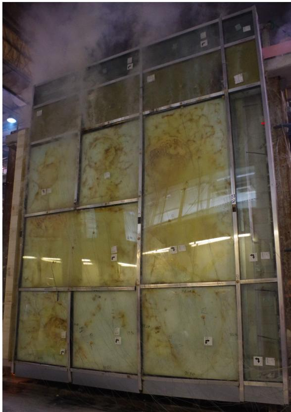
Fig. 37 Unexposed side of the test specimen,  $t = 67$  m
