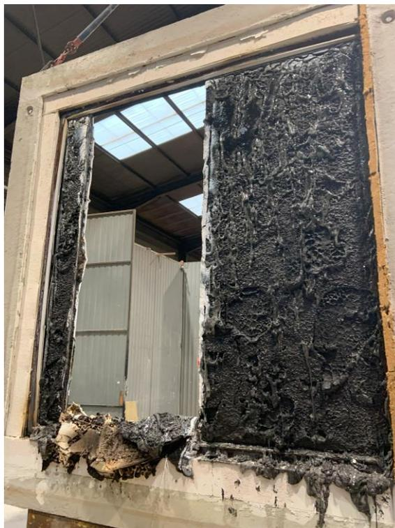
*Photo F: Exposed side of the element after the end of the fire test and the cool down of the element*
