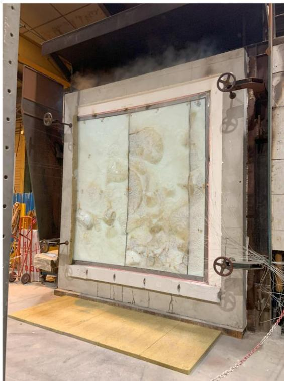
*Photo C: Non-exposed side of the element before the end of the fire test*
