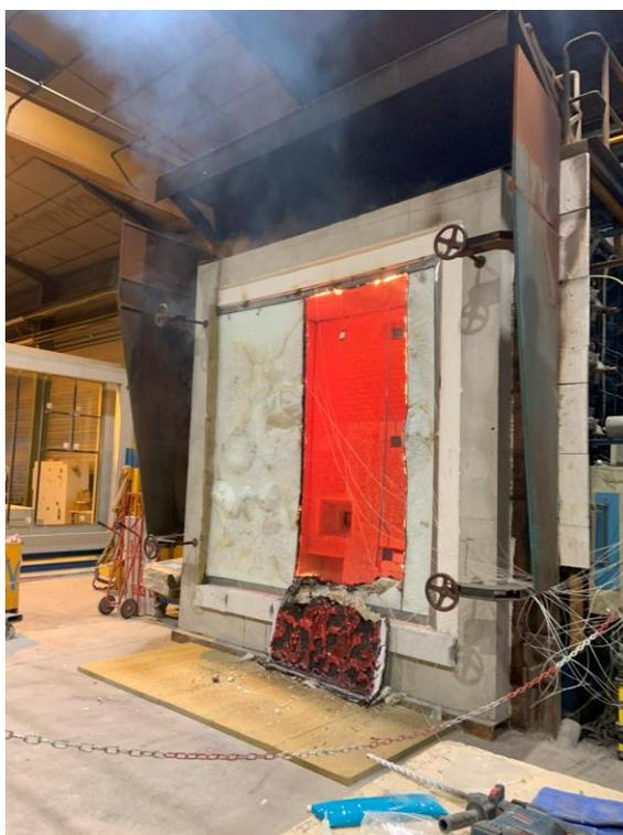
*Photo D: Non-exposed side of the element at the end of the fire test*
