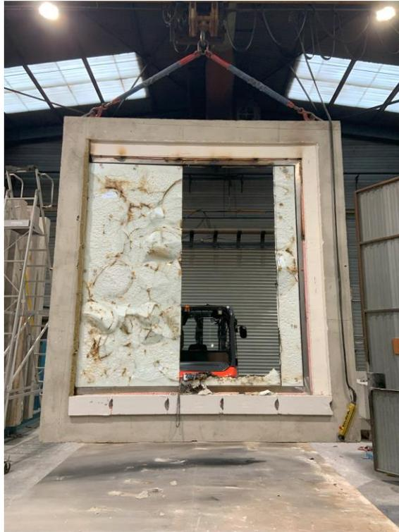
*Photo E: Non-exposed side of the element after the end of the fire test and the cool down of the element*
