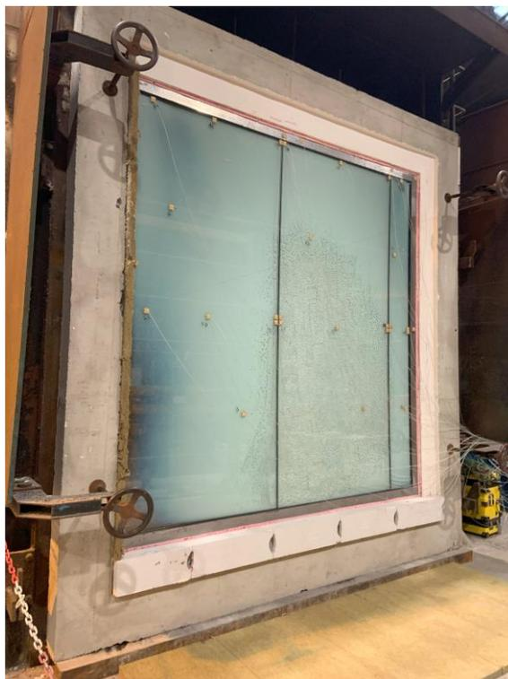
*Photo B: Non-exposed side of the element after the beginning of the fire test*
