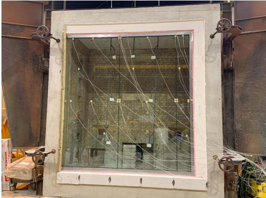
*Photo A: Non-exposed side of the element before the beginning of the fire test*
