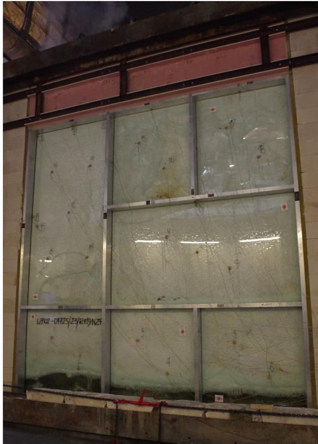
Fig. 27. Unexposed side of the test specimen,  $t = 61$  m
