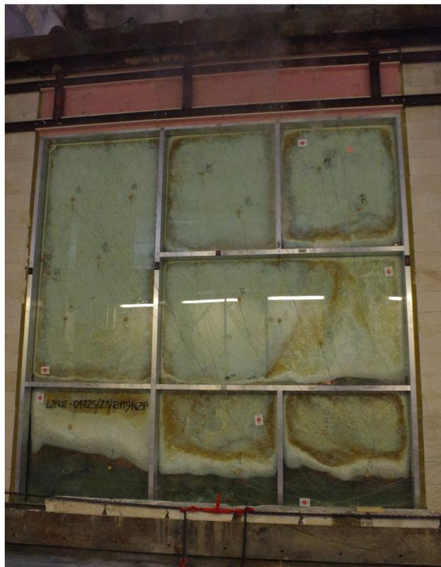
Fig. 25. Unexposed side of the test specimen,  $t = 15$  m
