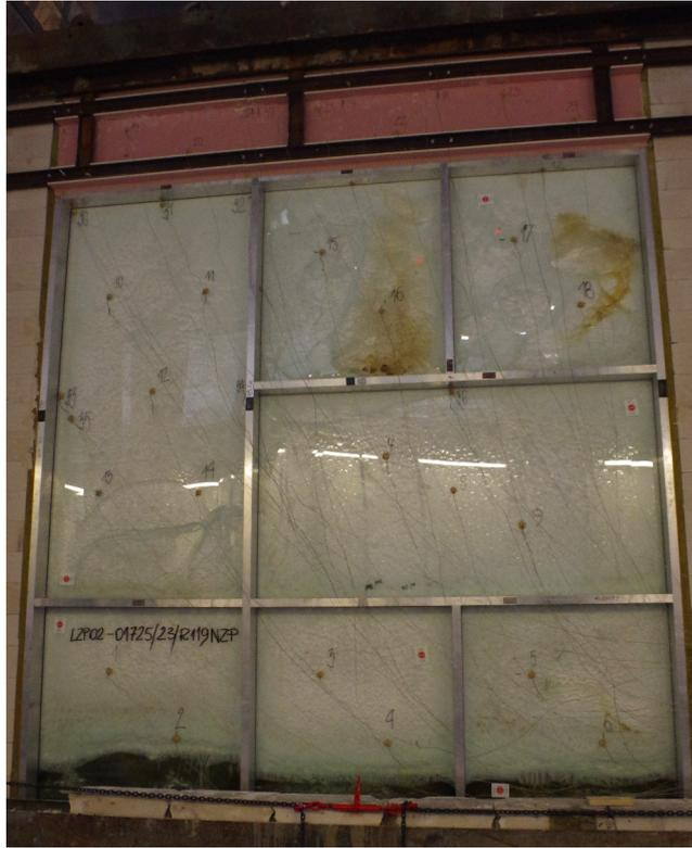
Fig. 28. Unexposed side of the test specimen after the test
