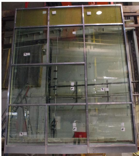
Fig. 1. Test specimen before the test – exposed side (before facing the furnace)
