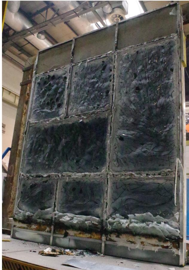
Fig. 29. Exposed side of the test specimen after the test
