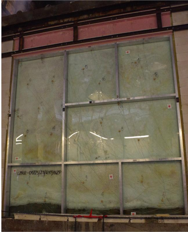
Fig. 26. Unexposed side of the test specimen,  $t = 41$  m
