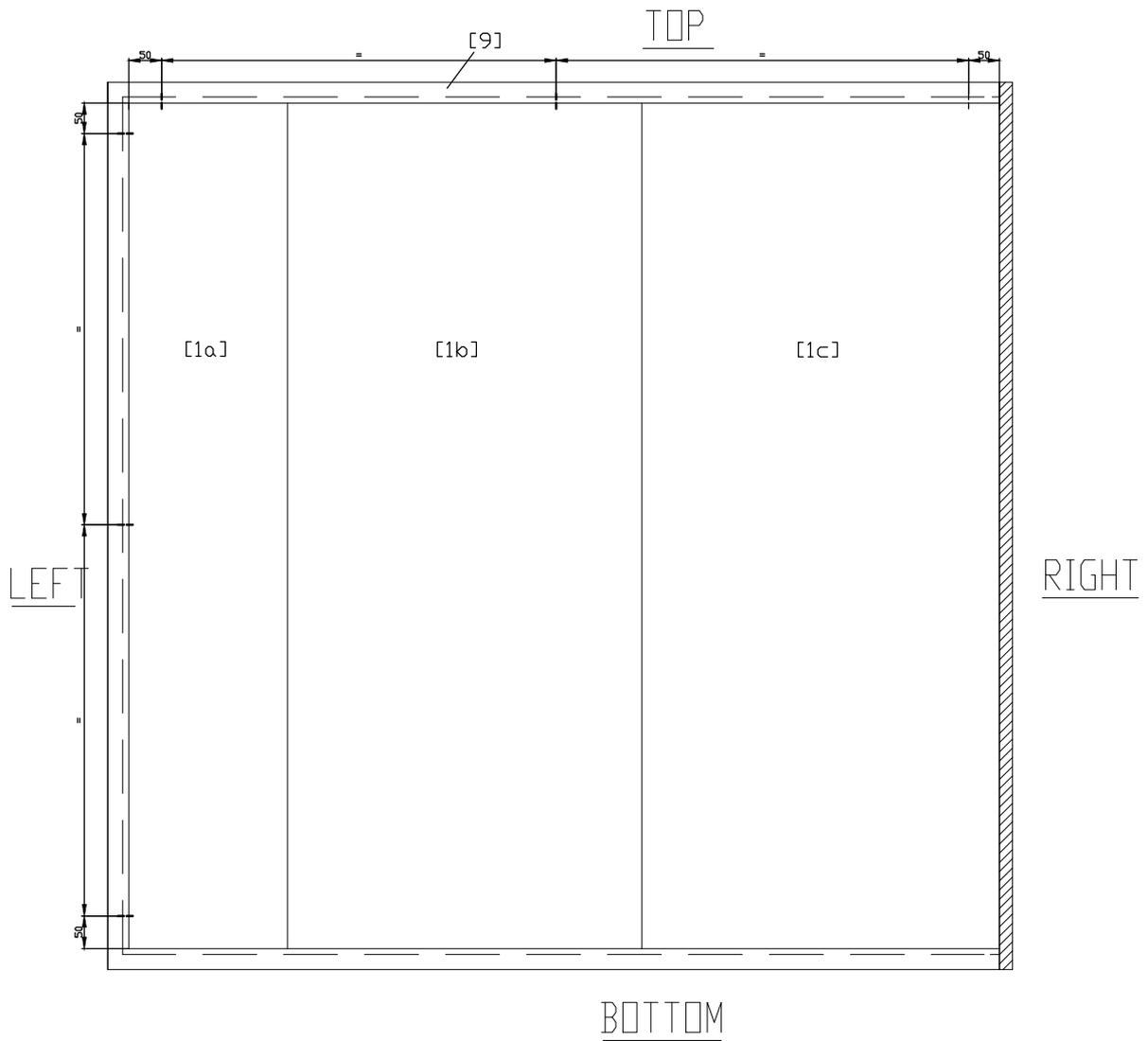
For glazing beads > 3 m => fixation with additional screws
