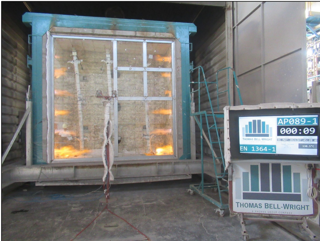
Picture 3: Unexposed face of the specimen after the commencement of the test.
