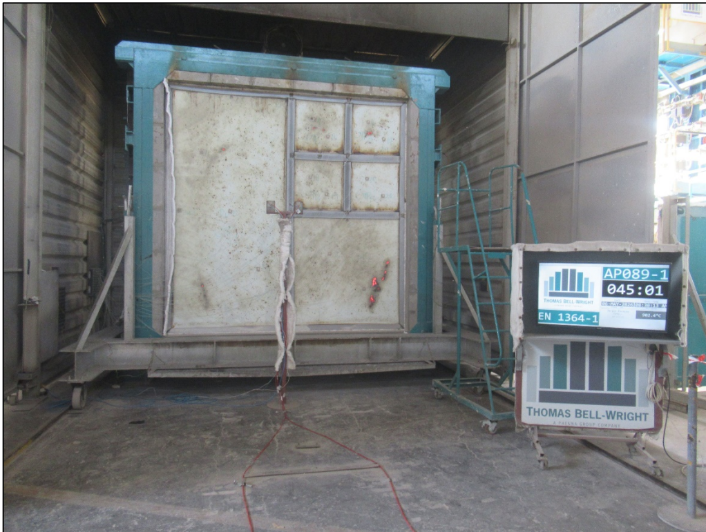
Picture 5: Unexposed face of the specimen after 45:00 minutes
