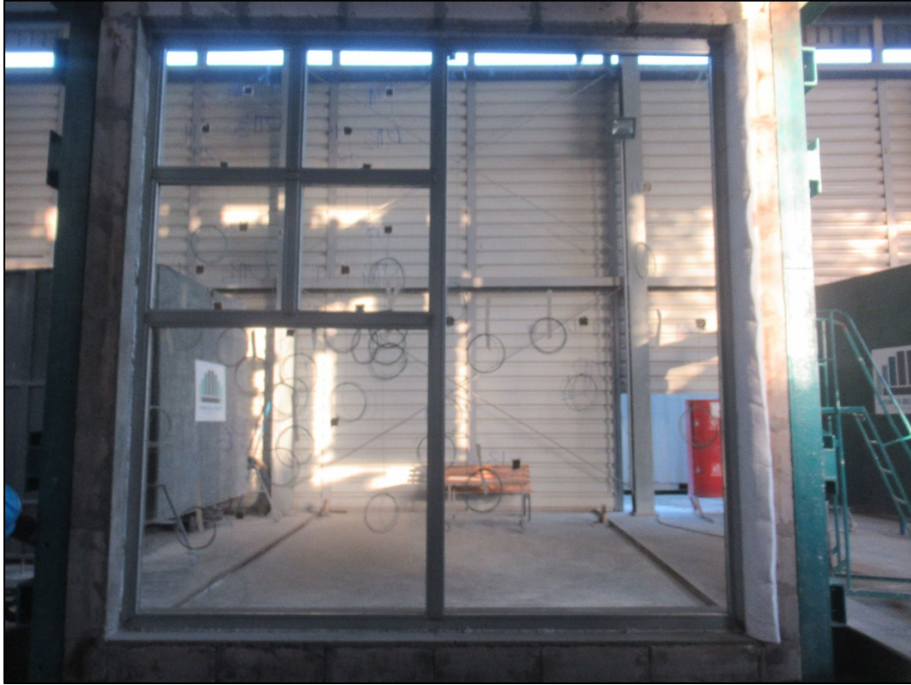
Picture 1: Exposed face of the specimen prior to the commencement of the test.
