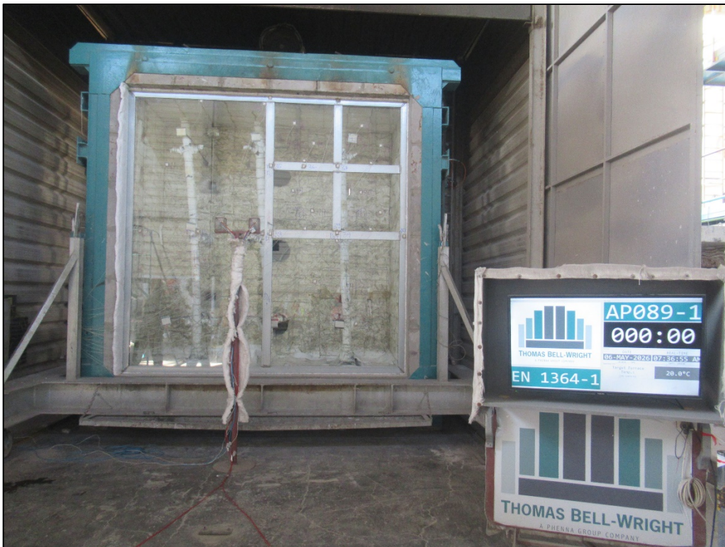
Picture 2: Unexposed face of the specimen prior to the commencement of the test.
