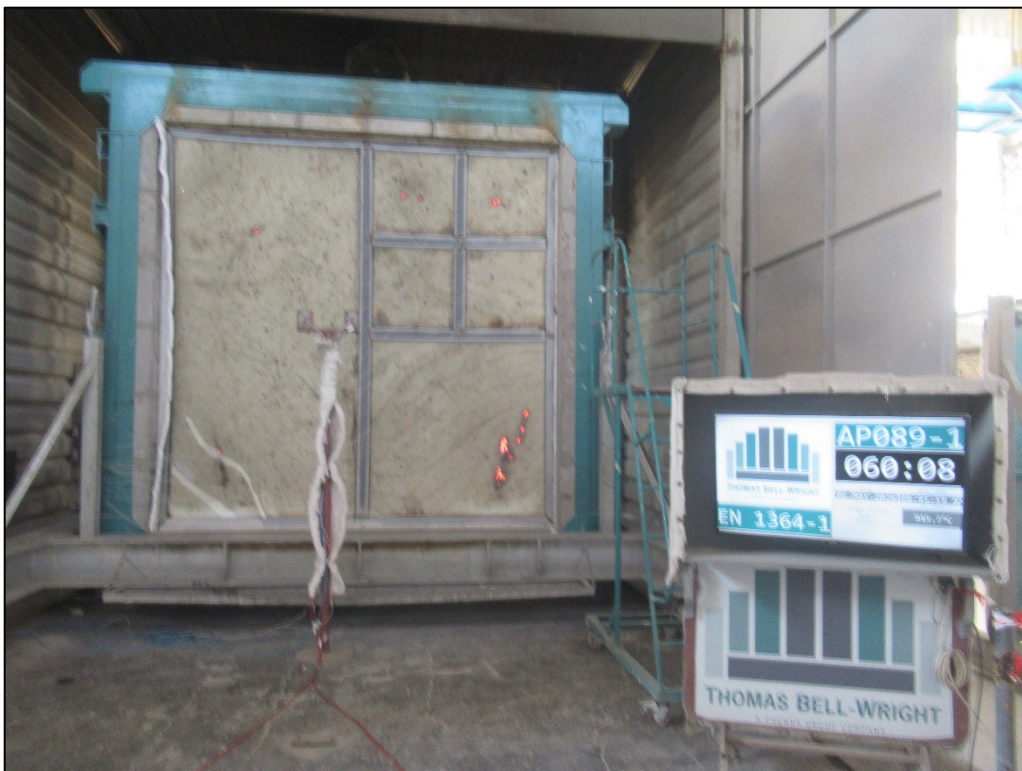
Picture 6: Unexposed face of the specimen after 60:00 minutes
