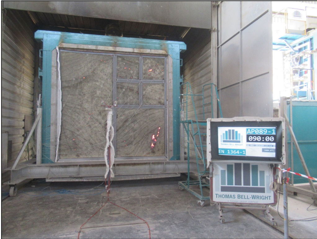
Picture 7: Unexposed face of the specimen after 90:00 minutes
