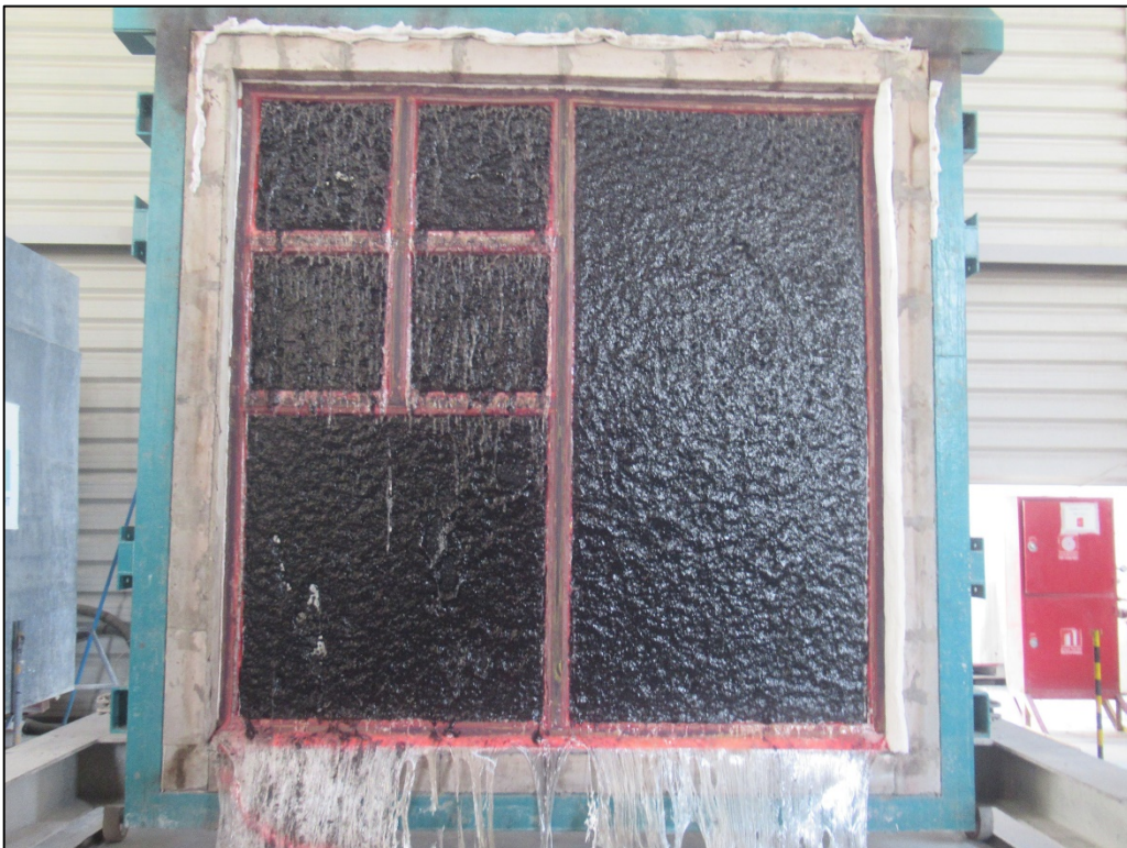
Picture 10: Exposed face of the specimen at the end of fire endurance test.
