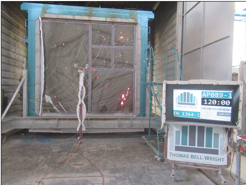
Picture 8: Unexposed face of the specimen after 120:00 minutes
