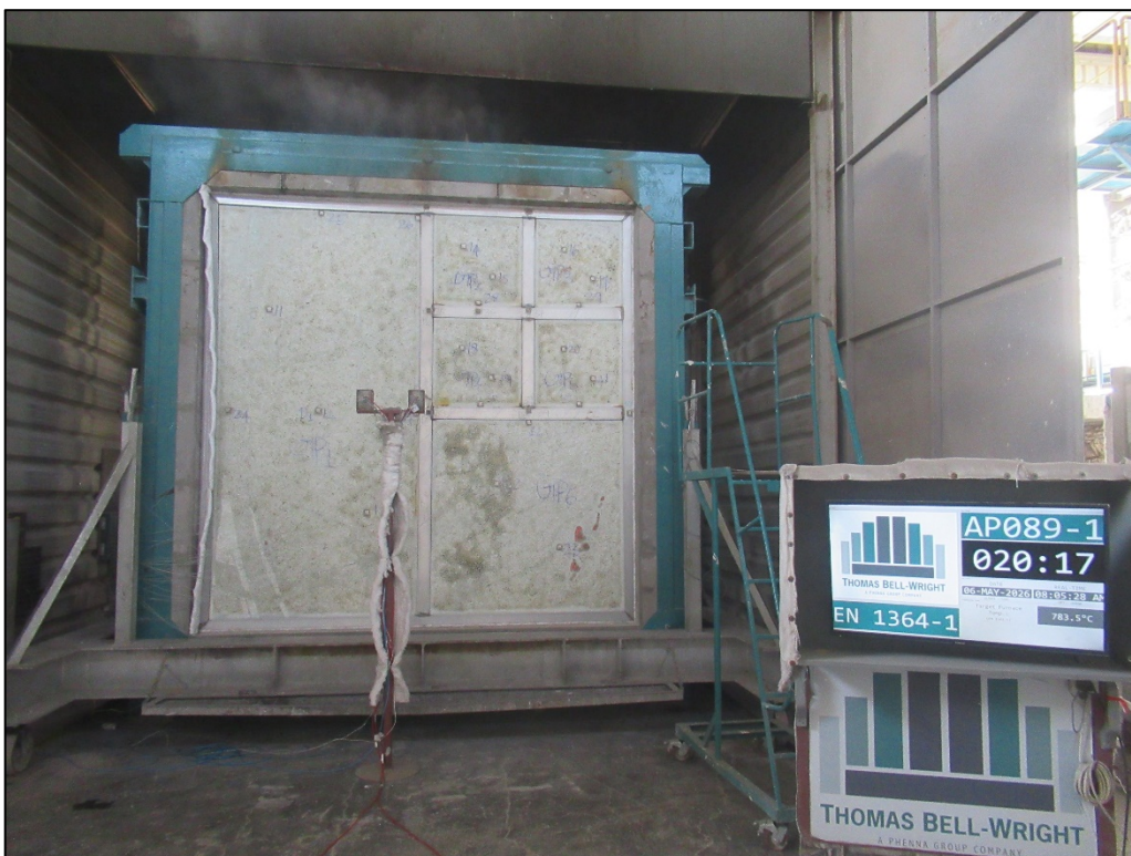
Picture 4: Unexposed face of the specimen after 20:00 minutes
