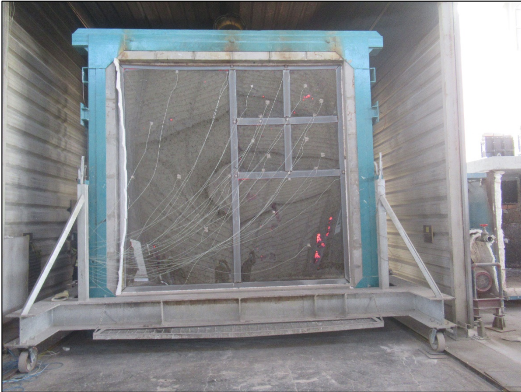
Picture 9: Unexposed face of the specimen at the end of the fire endurance test.
