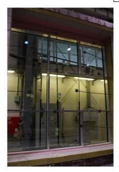
Fig. 1. Test specimen before the test – exposed side (before facing the furnace)
