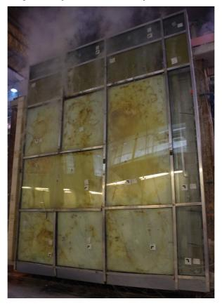
Fig. 37 Unexposed side of the test specimen, t = 67 m
