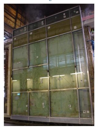
Fig. 33. Unexposed side of the test specimen, t = 10 m
