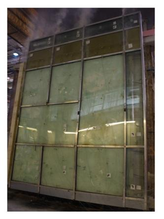
Fig. 35. Unexposed side of the test specimen, t = 45 m
