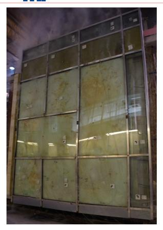
Fig. 36. Unexposed side of the test specimen, t = 61 m
