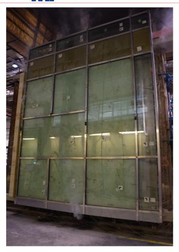
Fig. 34. Unexposed side of the test specimen, t = 31 m
