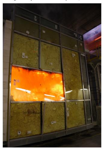
Fig. 35. Unexposed side of the test specimen after the test
