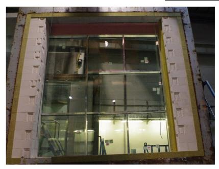
Fig. 1. Test specimen before the test – exposed side (before facing the furnace)
