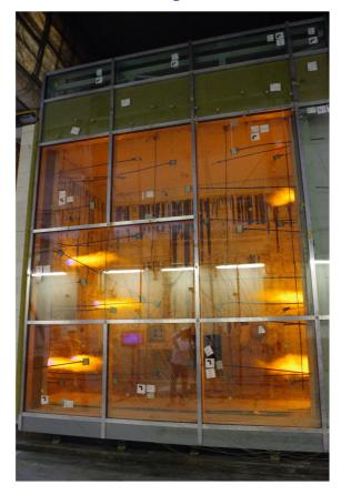
Fig. 32. Unexposed side of the test specimen, t = 16 m
