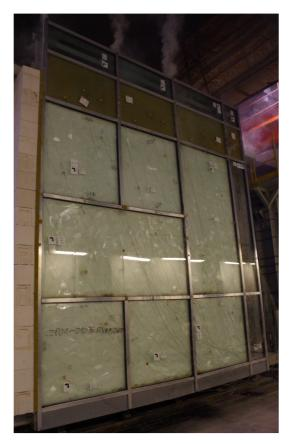
Fig. 33. Unexposed side of the test specimen, t = 31 m
