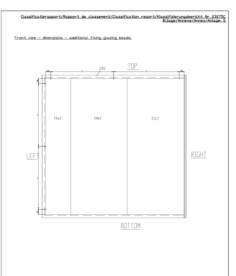
For glazing beads > 3 m => fixation with additional screws
