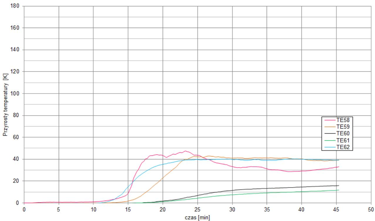
Fig. 26. Temperature rise on the unexposed surface of the test specimen – maximum temperature thermoelements
