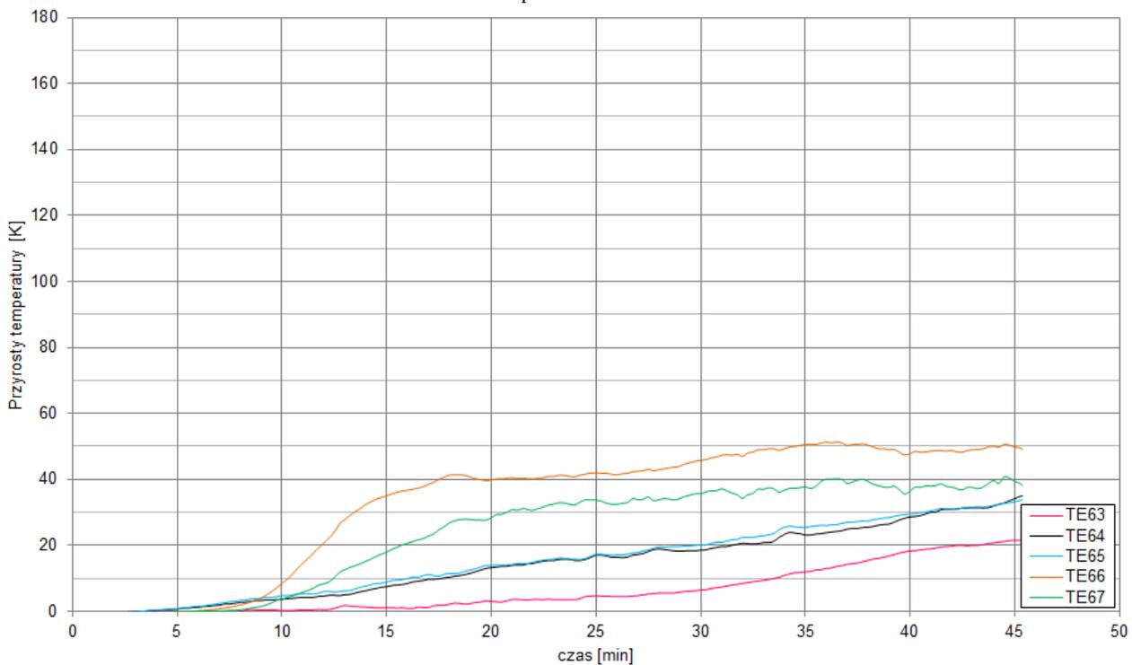
Fig. 27. Temperature rise on the unexposed surface of the test specimen – maximum temperature thermoelements
