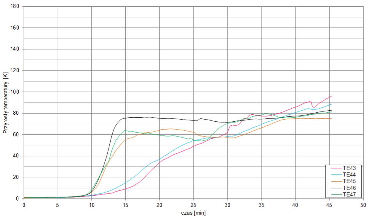
Fig. 23. Temperature rise on the unexposed surface of the test specimen – maximum temperature thermoelements
