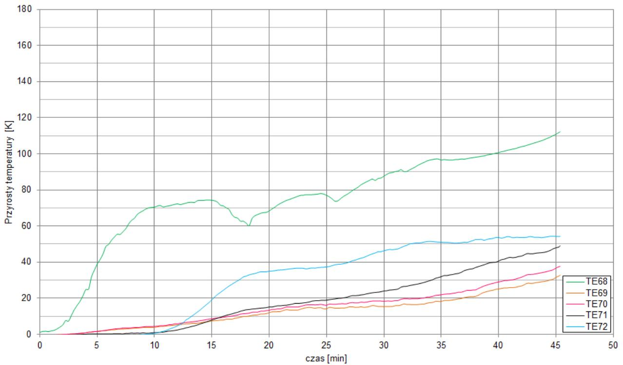
Fig. 28. Temperature rise on the unexposed surface of the test specimen – maximum temperature thermoelements
