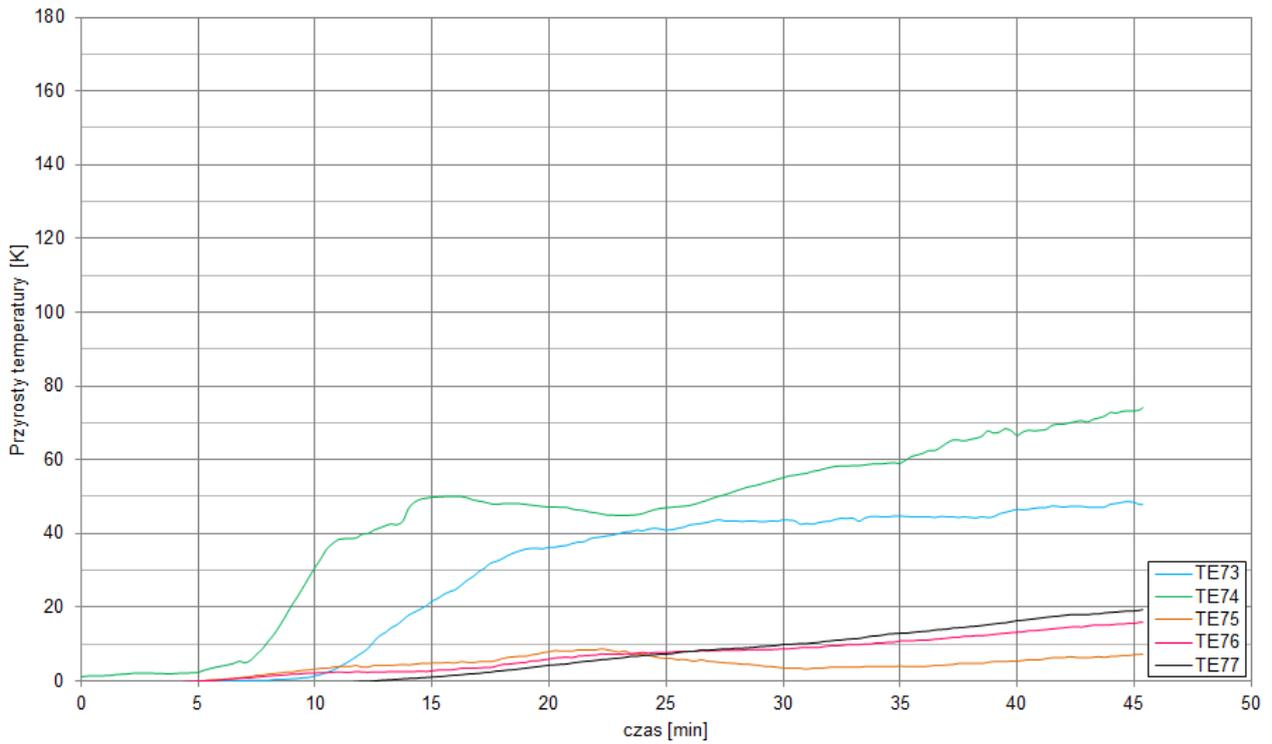
Fig. 29. Temperature rise on the unexposed surface of the test specimen – maximum temperature thermoelements
