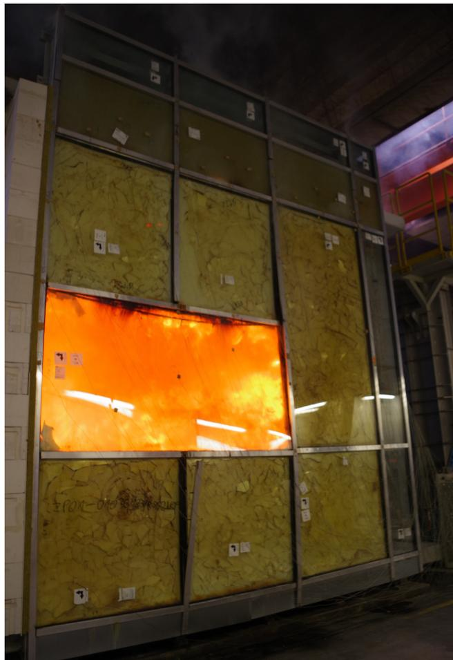
Fig. 35. Unexposed side of the test specimen after the test
