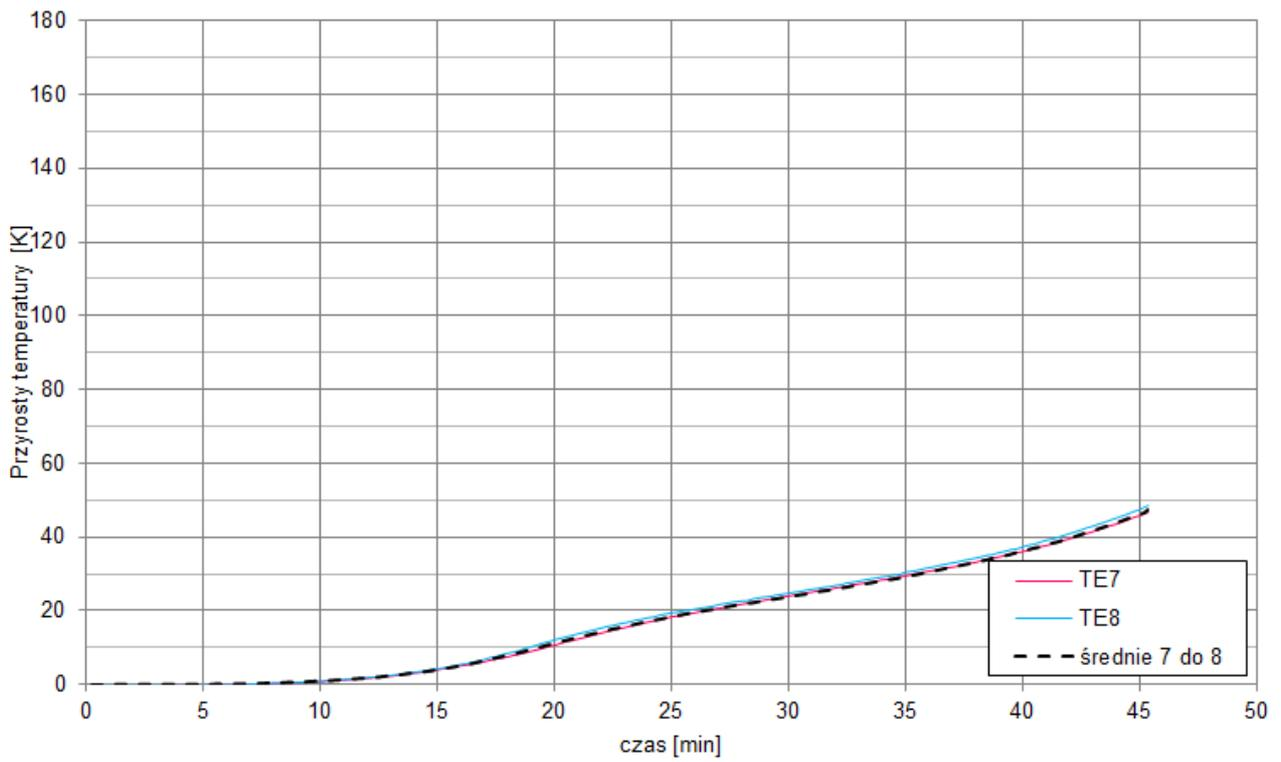
Fig. 12. Temperature rise on the unexposed surface of the test specimen - average and maximum temperature thermoelements
