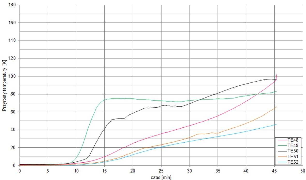
Fig. 24. Temperature rise on the unexposed surface of the test specimen - maximum temperature thermoelements
