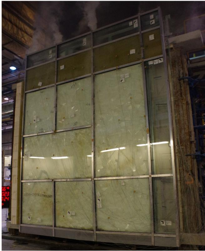
Fig. 34. Unexposed side of the test specimen,  $t = 45$  m
