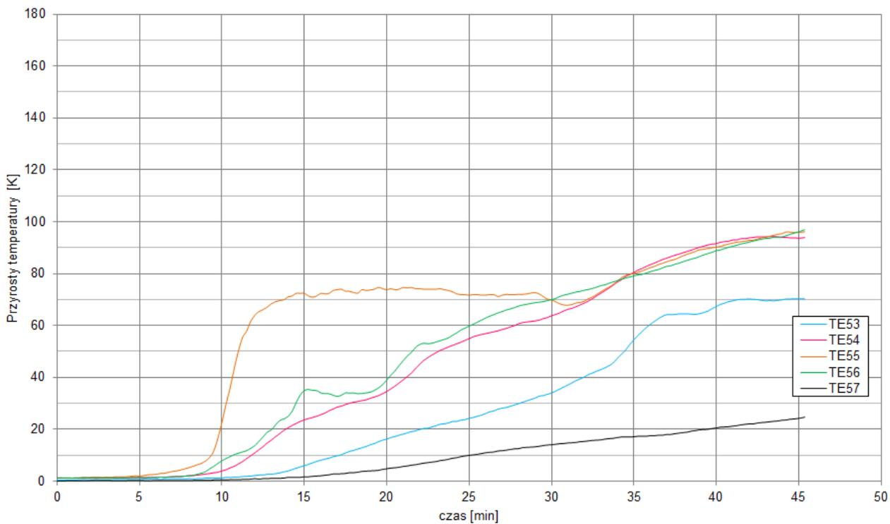
Fig. 25. Temperature rise on the unexposed surface of the test specimen - maximum temperature thermoelements
