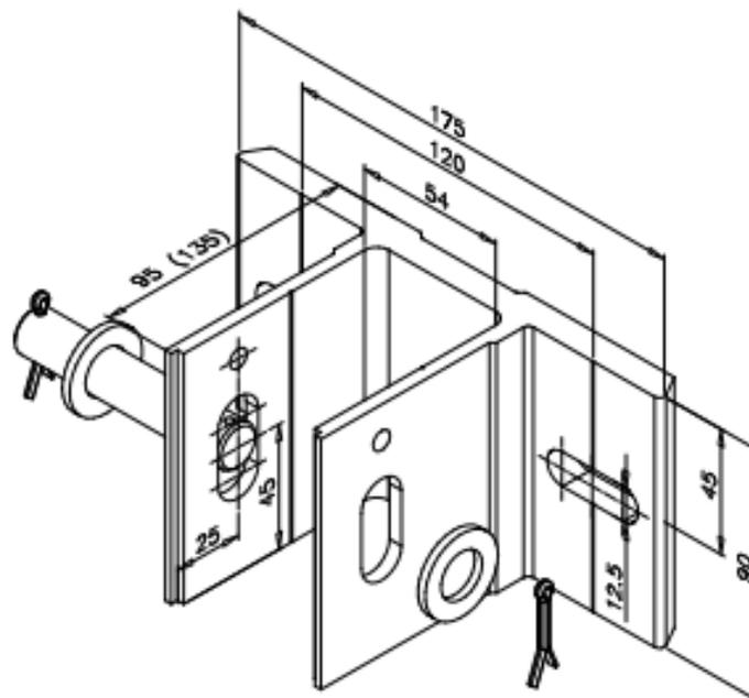
Rys. 19A. Sliding bracket cat. No. 80002128
