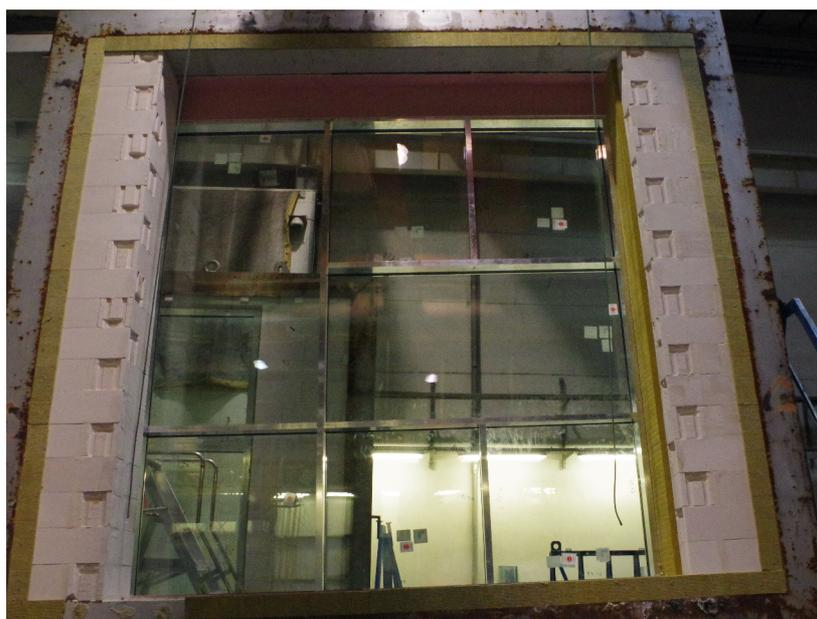
Fig. 1. Test specimen before the test – exposed side (before facing the furnace)
