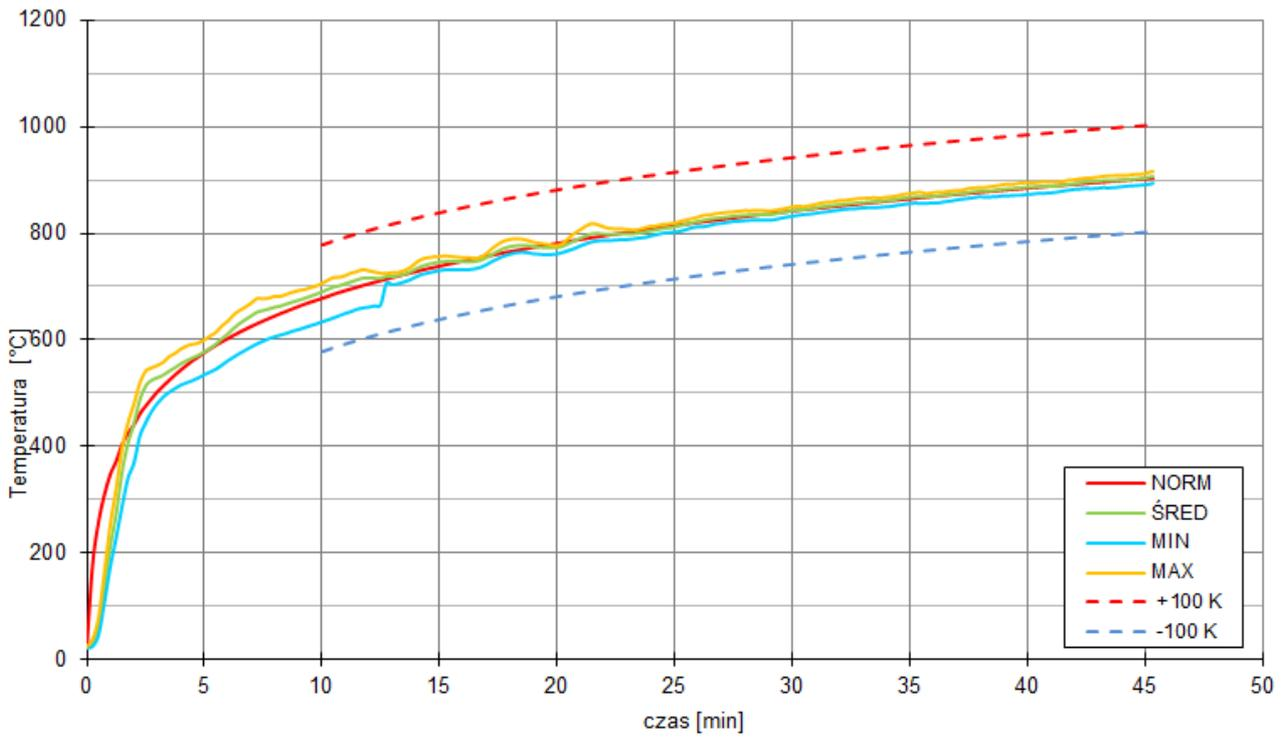
Fig. 5. Temperature of furnace heating conditions
