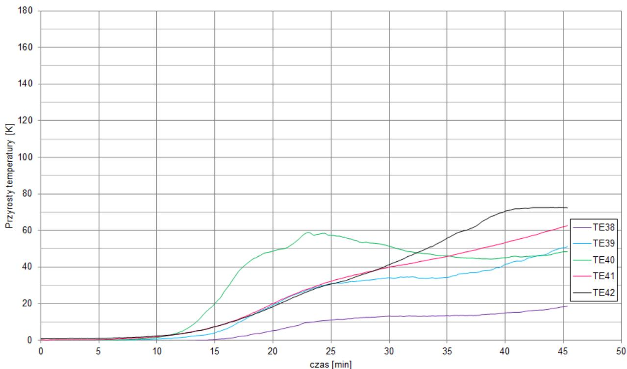
Fig. 22. Temperature rise on the unexposed surface of the test specimen – maximum temperature thermoelements
