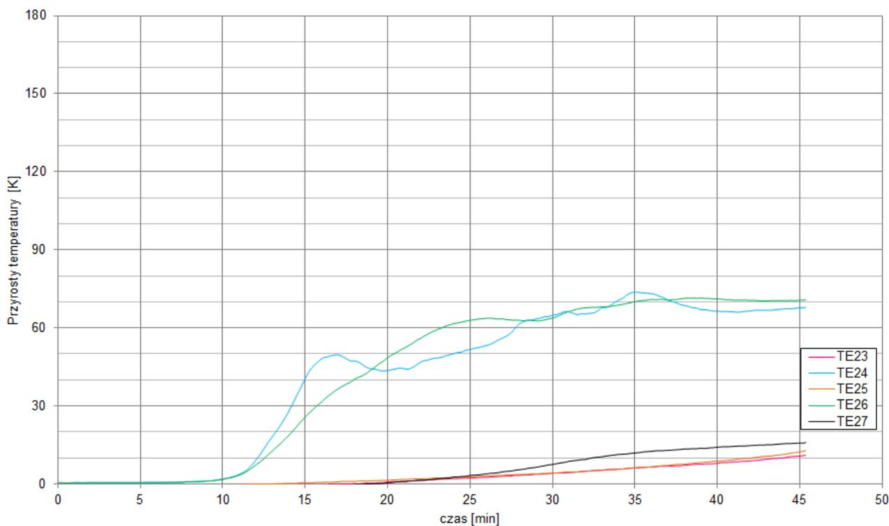
Fig. 19. Temperature rise on the unexposed surface of the test specimen - maximum temperature thermoelements
