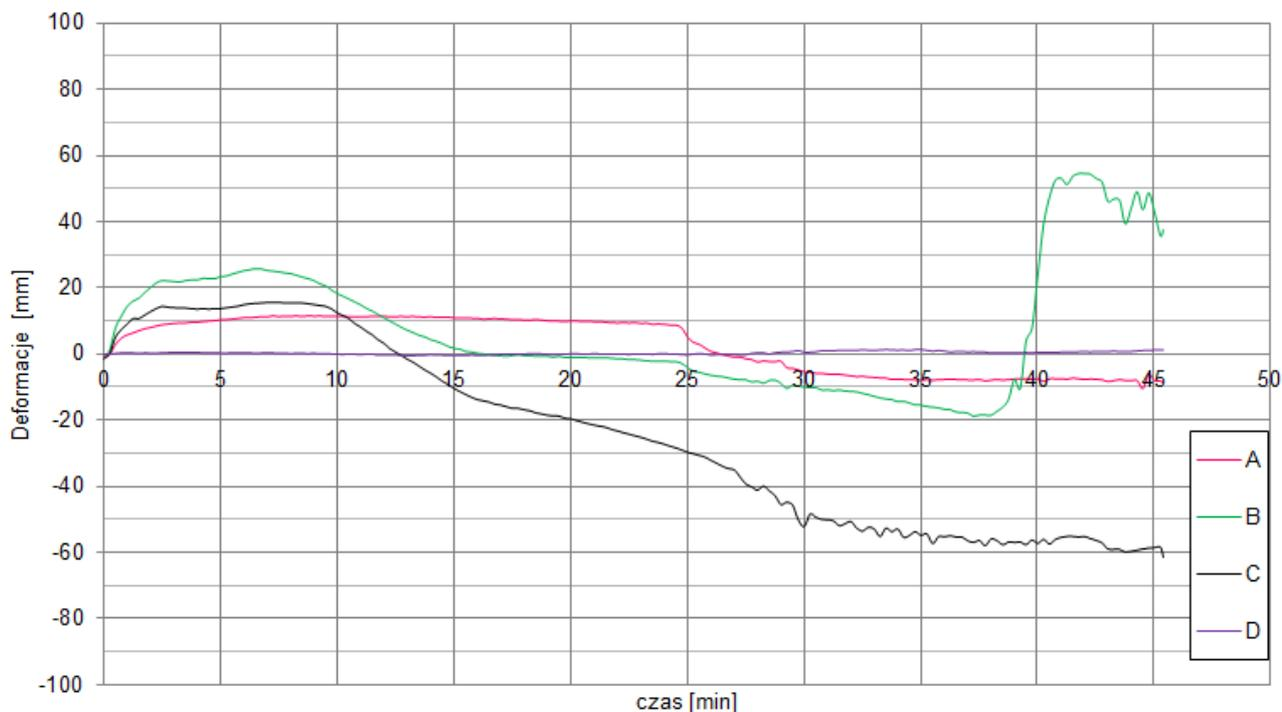
Fig. 31. Graph of deflections of the curtain wall perpendicular to its surface
