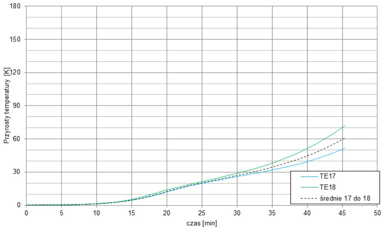
Fig. 16. Temperature rise on the unexposed surface of the test specimen - average and maximum temperature thermoelements
