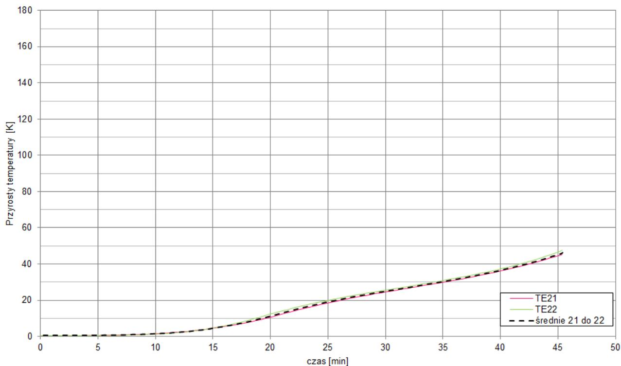
Fig. 18. Temperature rise on the unexposed surface of the test specimen - average and maximum temperature thermoelements
