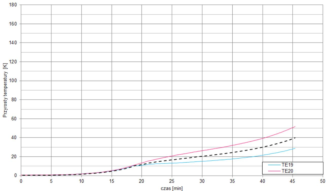
Fig. 17. Temperature rise on the unexposed surface of the test specimen - average and maximum temperature thermoelements
