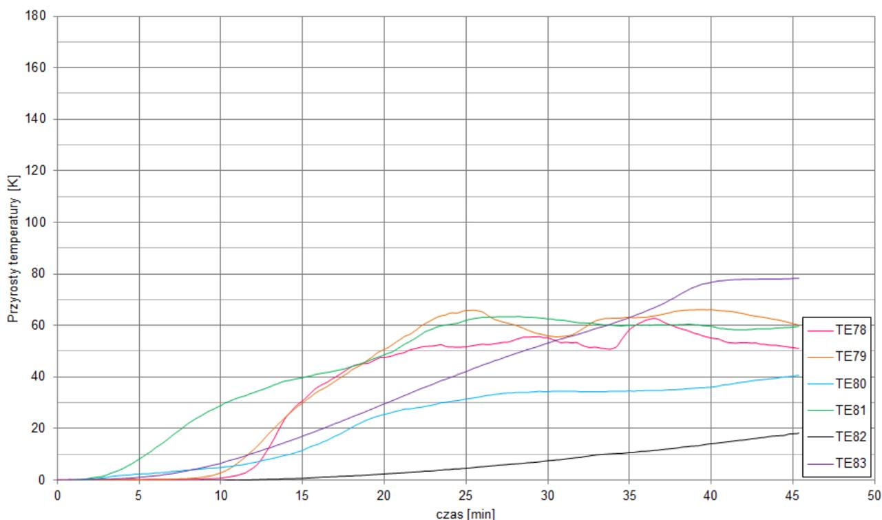
Fig. 30. Temperature rise on the unexposed surface of the test specimen – maximum temperature thermoelements
