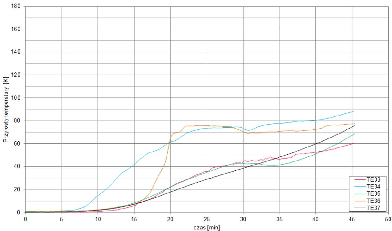
Fig. 21. Temperature rise on the unexposed surface of the test specimen – maximum temperature thermoelements
