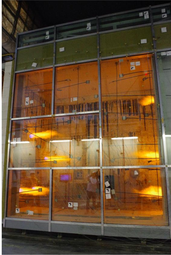
Fig. 32. Unexposed side of the test specimen,  $t = 16$  m
