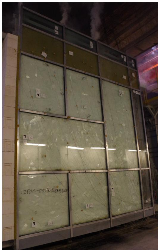
Fig. 33. Unexposed side of the test specimen,  $t = 31$  m
